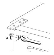
Unscrew the handle. Refit it on the opposite side after having pushed in the plugs with a punch. Cover the holes left open with the plugs contained in the documentation pack.
